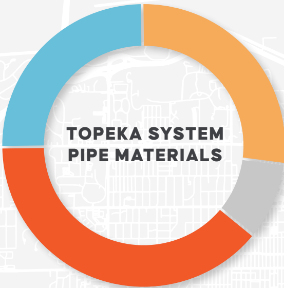
Fig. 1: Topeka's pipe system is 39% cast iron, 27% ductile iron, 25% PVC, with the remaining made of various other materials.
