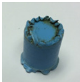
Coupons Showing “Crown” at Outer Surface
