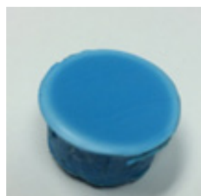
Coupons Showing “Punch-Through” at Inner Wall
