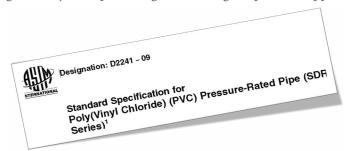
The body of the standard includes IPS (Iron Pipe Size) ODs, while an annex includes Plastic Irrigation Pipe (PIP) and Copper Tube Size (CTS) ODs. Currently there is a project under way at ASTM to add Cast Iron Pipe Size (CIPS) to the annex.
