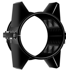
Model CSP Polyethylene Casing Spacer, high-density injection molded with a variety of runner heights available to allow for different carrier/casing profiles
